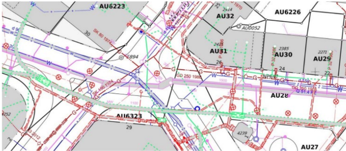
Figure 7. Multi-utility asset planning map and data provided in the City of Zürich, which includes gas, electricity; sewage; district heating; communication. 5
