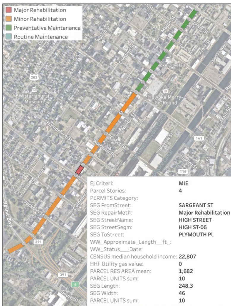
Figure 23. The Web-Hosted Digital Network Asset Registry displays Sargeant Street in Holyoke, MA.
