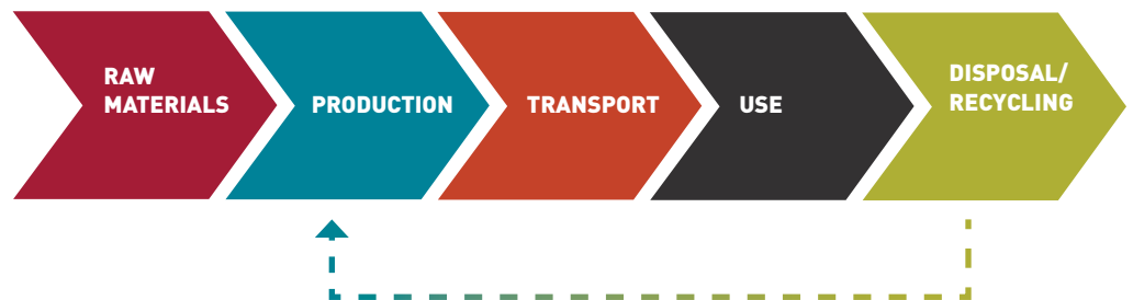
Figure 6. Diagram of a product life cycle. The dotted line connecting the “end-of-life” box with production indicates recycling.
